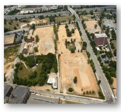
Abatement and Recycling of 71 structures totaling 450,000 SQ/FT; *Crushing screening and recycling of 29,000 tons of concrete.* 120 calendar days, \$2,400,000.
